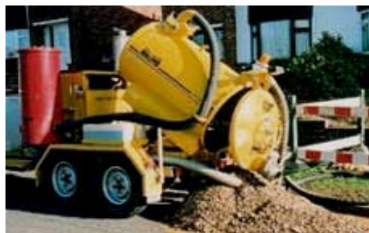
Top: Vacuum Excavation limits space requirements.
