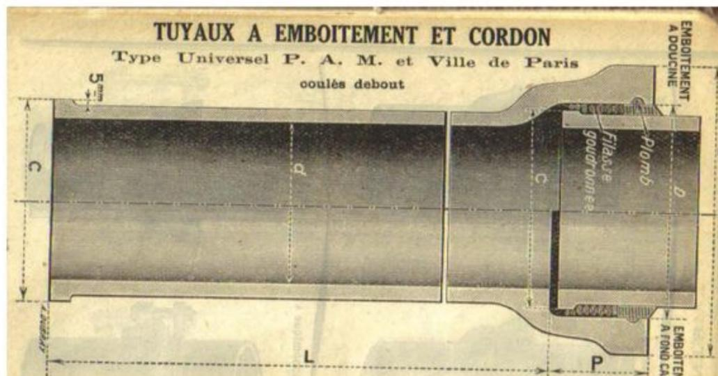
Figure 1. Gray cast iron pipe with bell and spigot and with lead caulked joint. Extract from the 1920 Pont-à-Mousson catalog.
