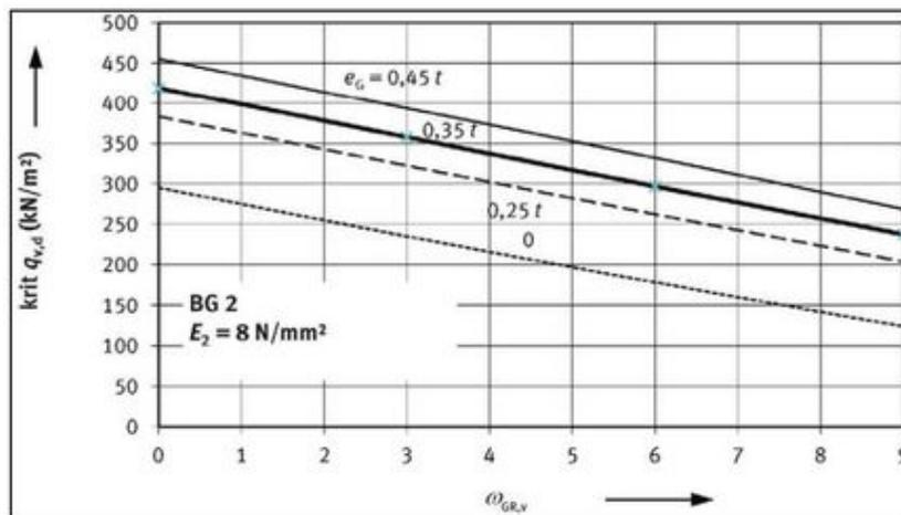
Figure 5. Critical vertical loads of the fourfold cracked host pipe, soil group G2,  $K_2 = 0.3$ ;  $E_2 = 8 \text{ N/mm}^2$  [DWA-A 143-2, Diagram F.4].
