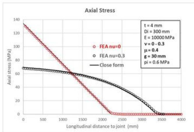
Figure 6. Axial stress versus longitudinal distance to joint and Poisson's coefficient.
