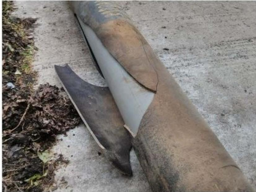
**Figure 8. Fractured gas host pipe after loading in pit test and integer SAERTEX-LINER® GAS**
