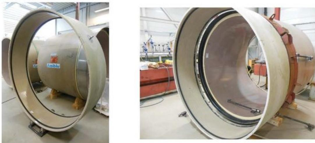
**Figure 6. External sleeve for pressure application**
