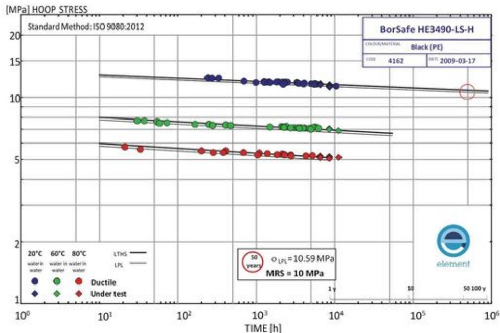
Figure 2. 50-year extrapolation in Element test report P-09/38-v2.
