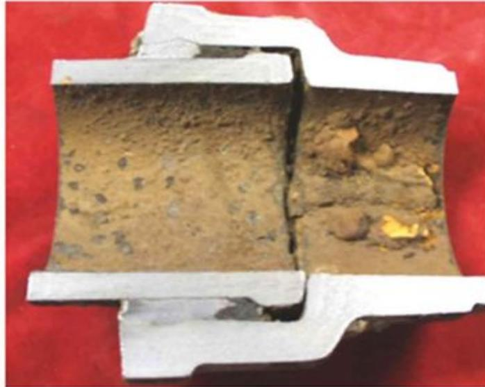
Figure 6. Gap in spigot and socket joint.
