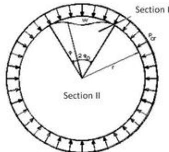
Figure 7. Pipe-in-pipe model [Glock, 1977].
