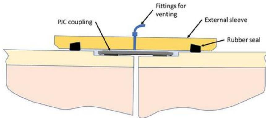
**Figure 5. Method for applying external pressure on joint**
