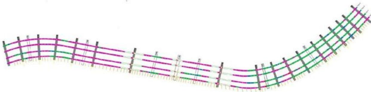
Fig.4: planimetric diagram of the pipes inside the bridge, with indication of the measured thicknesses
