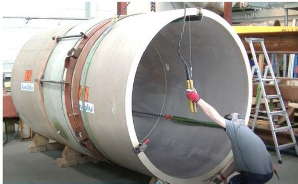
**Figure 7. Assembly and adjusting angular deflection**
