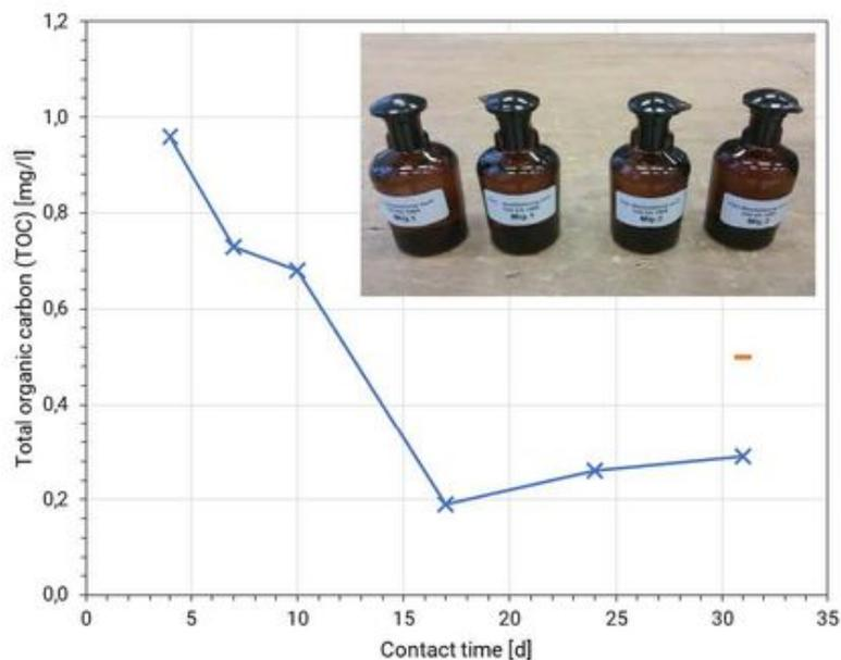
Figure 4. Data set of SAERTEX-LINER® H2O, measurement of TOC in contact water with time
