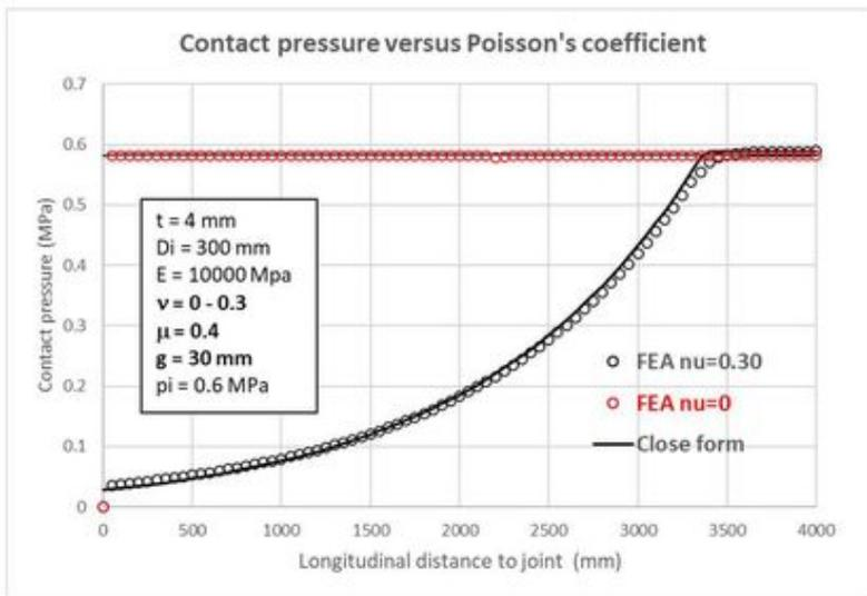
Figure 8. Contact pressure versus longitudinal distance to joint and Poisson's coefficient.
