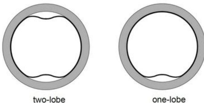
Figure 2. Typical buckling modes.
