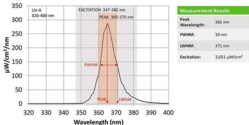
Figure 1: UV Spectrum of different wave lengths
