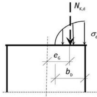
Figure 6. Parabolic stress distribution in the contact zone of longitudinal transom cracks [DWA-A 143-2].
