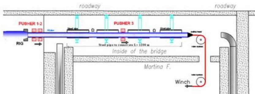
Fig.8: Installation scheme
