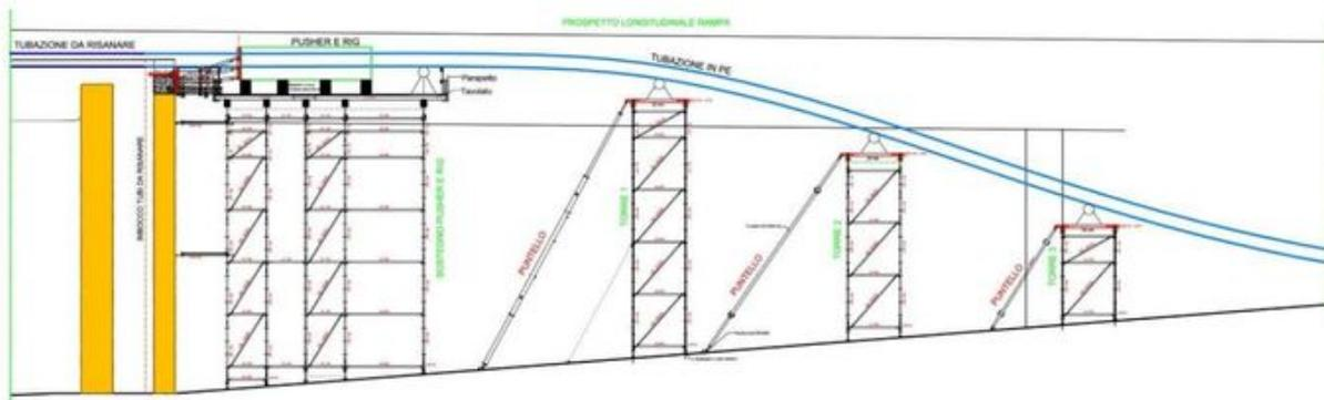
Fig 11: longitudinal profile of the insertion ramp
