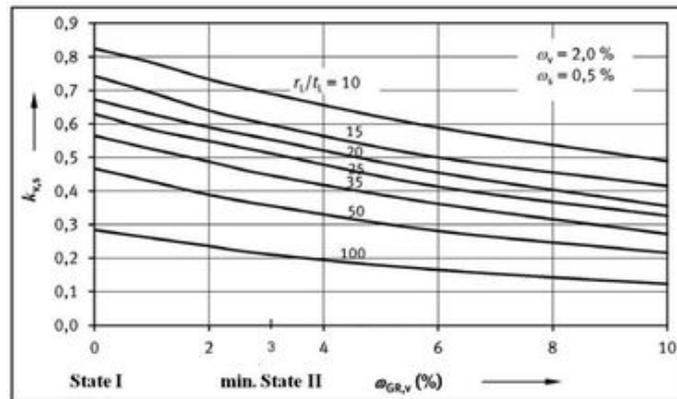
Figure 9. Diagram for determining  $k_{v,s}$  as a function of the joint ring deformation  $w_{GR,v}$  [DWA-A 143-2].
