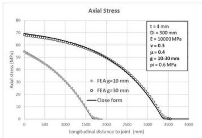
Figure 5. Axial stress versus longitudinal distance to joint and gap.
