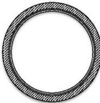
Figure 3. Liner constrained by the host pipe
