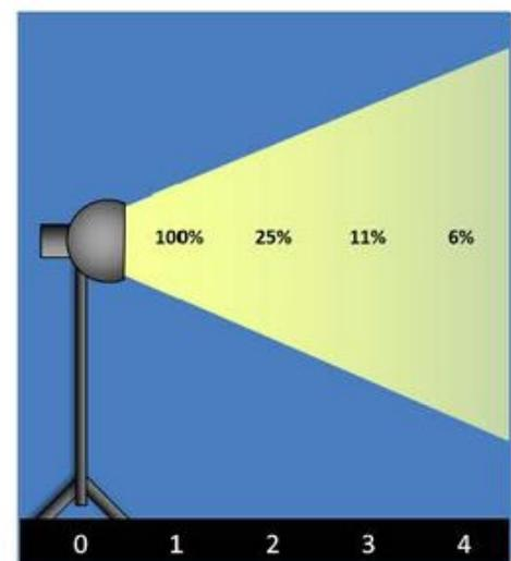
Figure 3: Drop of UV-light intensity
