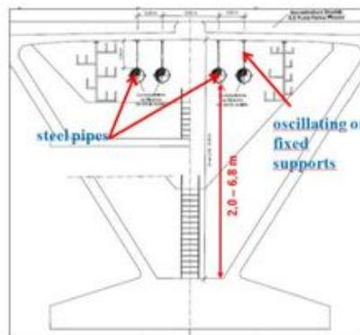
Fig.3: bridge section
