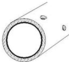
**Figure 5. Class B, interactive semi-structural liner.**
