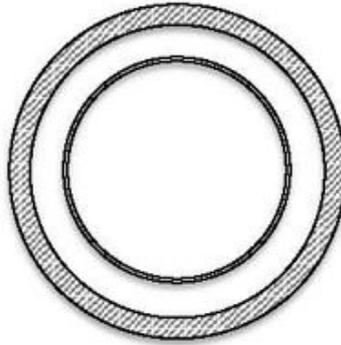
Figure 2. Liner unconstrained by the host pipe
