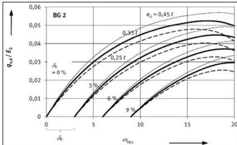
Figure 4. Load-displacement curves of the fourfold cracked host pipe for  $q_{v,d}$ , soil group G2,  $K_2 = 0.3$  [DWA-A 143-2, Diagram F.3].
