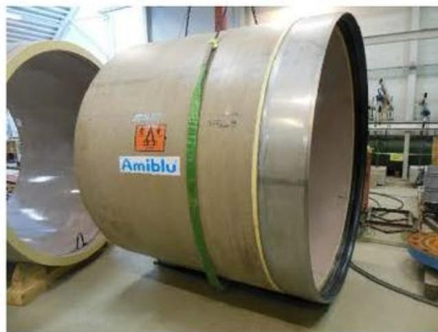
**Figure 4. Test pipe with mounted PJC coupling**
