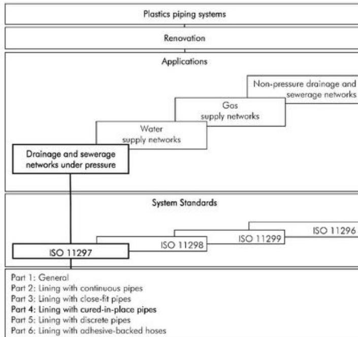
**Figure 1. CIPP product and standardization family, diagram from EN ISO 11297-4**
