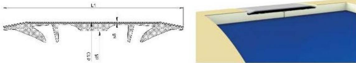
**Figure 3. Pressure Jacking Coupling (PJC) cross section and assembly**
