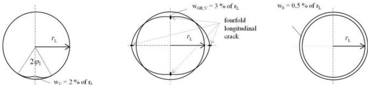
Figure 8. Local imperfection  $w_v$ , joint ring deformation  $w_{GR,v}$  and annular gap  $w_s$  [DWA-A 143-2].
