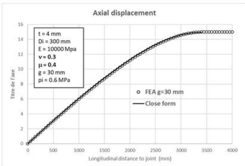
Figure 9. Axial displacement.
