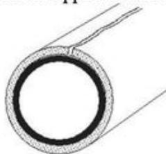
**Figure 4. Class A, independent fully structural liner.**
