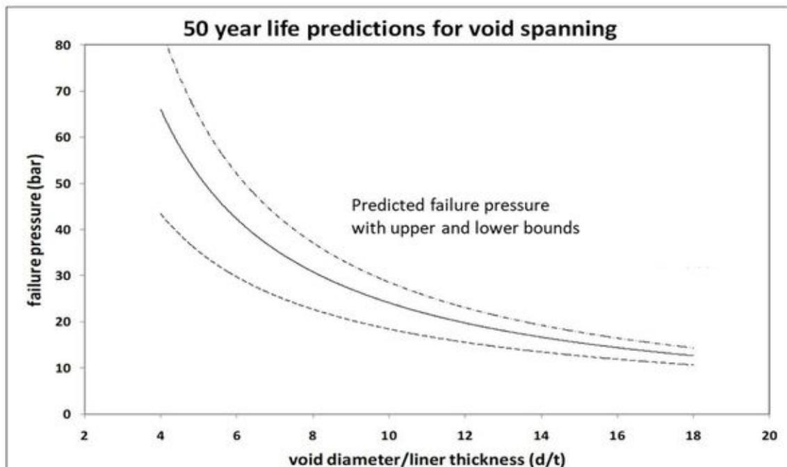
Figure 7. 50-year life void/hole spanning predictions for a PE 80 lining.
