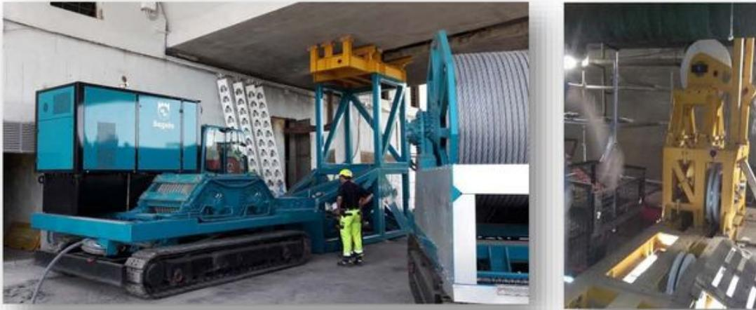
Fig.13: The winch, with a pulling capacity of 100 t - system of ropes and rollers
