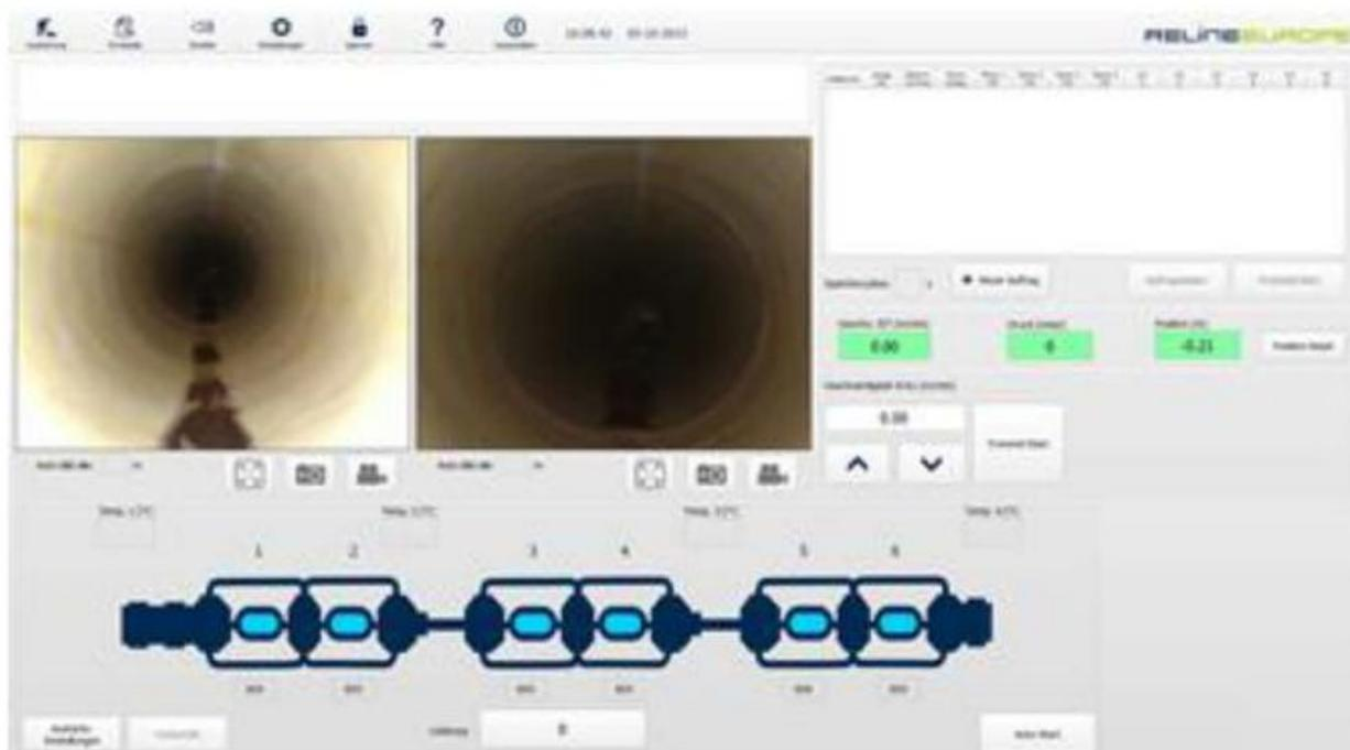
Figure 7: Real-time monitoring of the whole curing process
