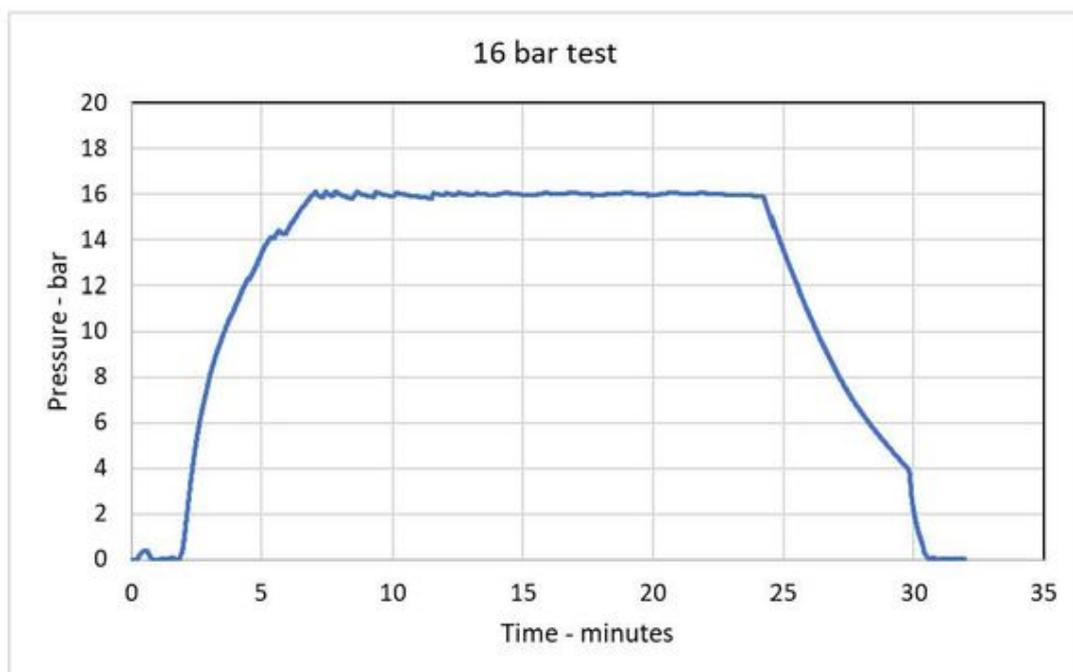
**Figure 11. Fifteen minutes 16 bar test**
