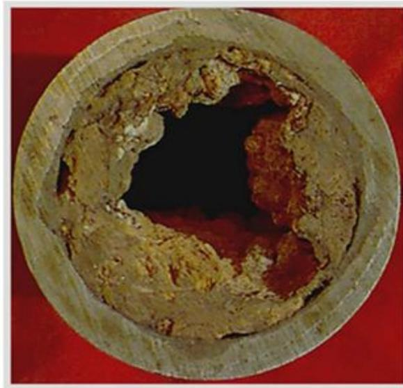
**Figure 1. Small diameter cast iron water pipe showing reduced flow capacity due to tuberculation.**
