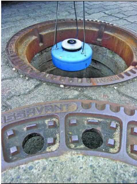
Figure 4.2. Panoramo® manhole inspection camera. https://www.mswmag.com/g/wef-tec-product-preview/2015/08/rapidview_ibak_north_america_panoramo_si
