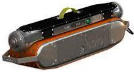
Figure 3.20. Autonomous crawler. https://www.redzone.com/
