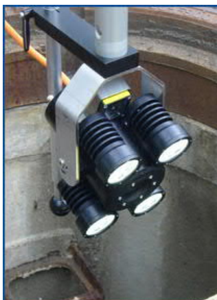
Figure 3.7. A zoom-camera. https://www.messen-nord.de/products/drain-testing-and-inspection/drain-testing-and-inspection-manhole-camera-systems.html?L=1
