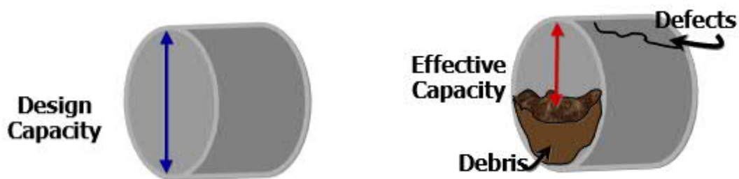
Figure 1.2. Illustration of the effective capacity and design capacity of a pipeline (Rowe et al. 2004).
