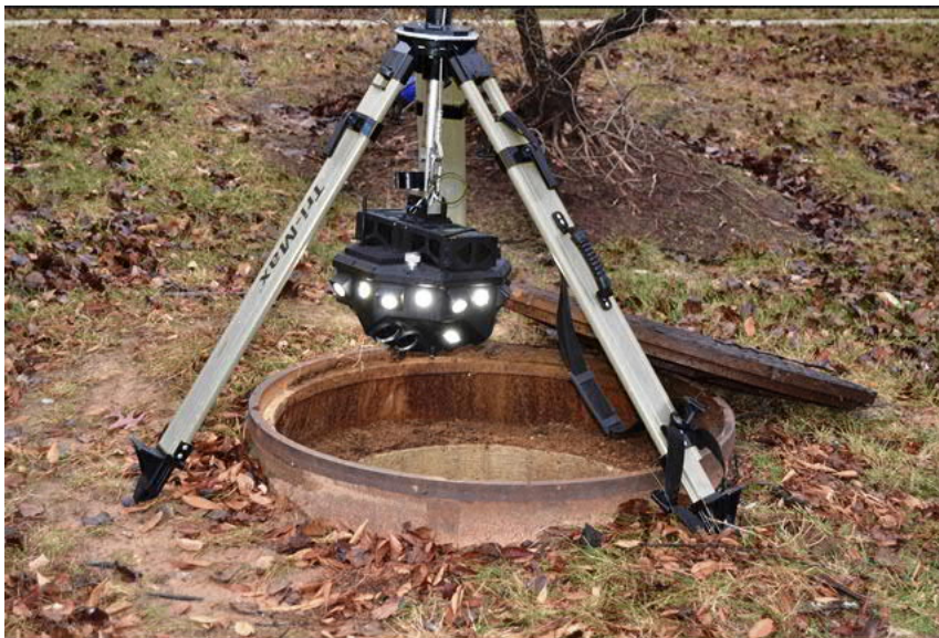
Figure 4.3. 3D color manhole scanning equipment. https://trenchlesstechnology.com/cues-introduces-first-wireless-3d-color-manhole-scanning-technology/
