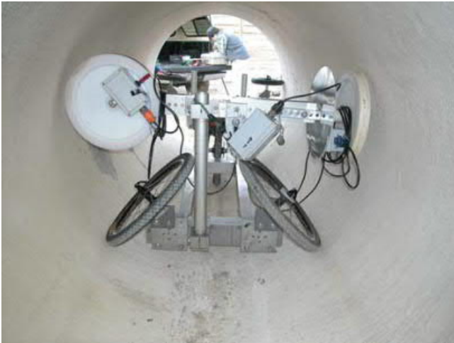
Figure 3.25. Magnetic field inspection robot. https://puretechltd.com/technology/purero-botics-pipeline-inspection-system/
