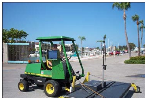
CART Array comprises 17 antennae (9 transmitters and 8 receivers)
