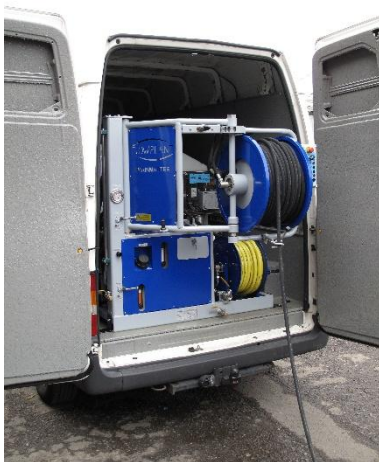
A van-mounted High Velocity (or Water Jet) cleaning unit. Picture courtesy of Flowplant.
