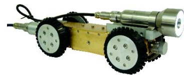
Typical CCTV camera systems used for non man entry pipeline surveys. Pictures courtesy of AM Industrial.
