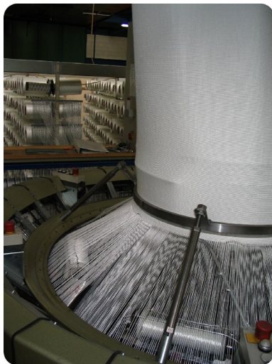
Woven Hose Liner Circular Weaving system
