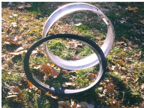
Internal connection seal and backing ring (left) and (right) Seal fitted and expanded.
