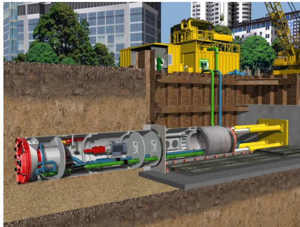
A typical re-circulating slurry system arrangement for a microtunnelling machine. Picture courtesy of Herrenknecht.
