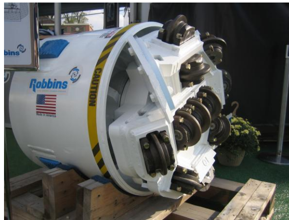
An SBU unit for use with auger boring systems. Picture courtesy of Robbins and U Mole.
