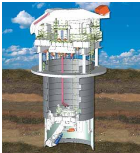
A schematic of the operation of a shaft sinking rig. Picture courtesy of Herrenknecht AG
