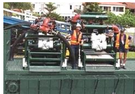
A typical HDD fluid recycling set-up. Picture courtesy of Kem-Tron Inc
