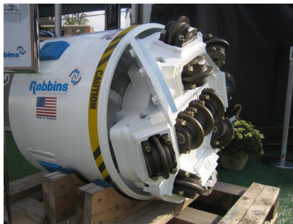
An SBU small diameter cutter head for rock conditions. Picture courtesy of U Mole/Robbins.
