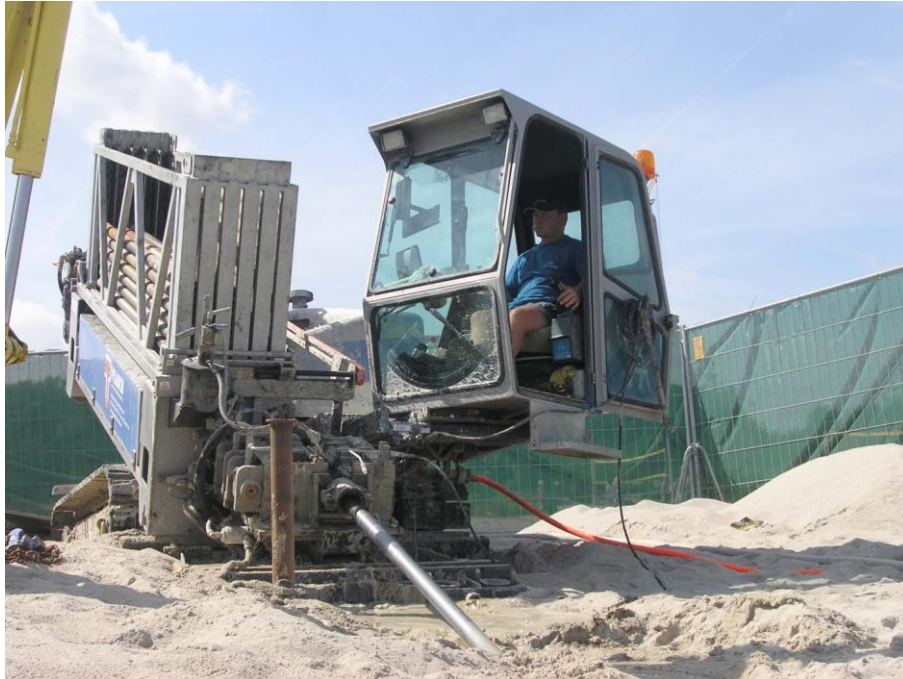
A surface-launched horizontal directional drilling rig. Picture courtesy of Tracto-Technik.
