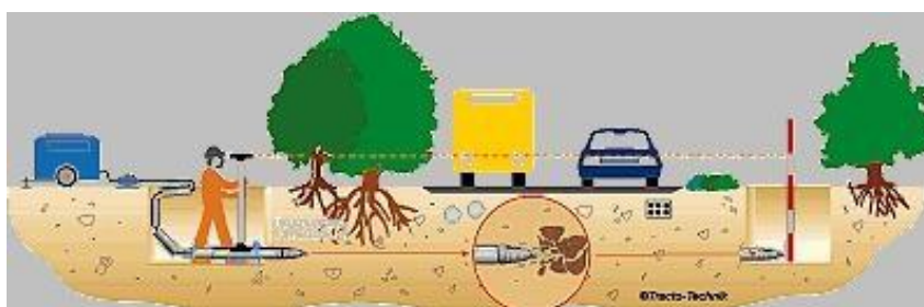
Schematic of the Impact Moling process.
