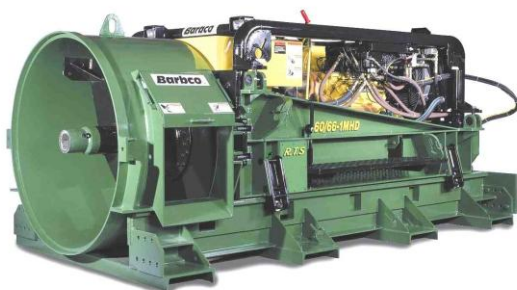
Typical Auger Boring machines. Pictures courtesy of Barbo (left) and American Augers (right)
