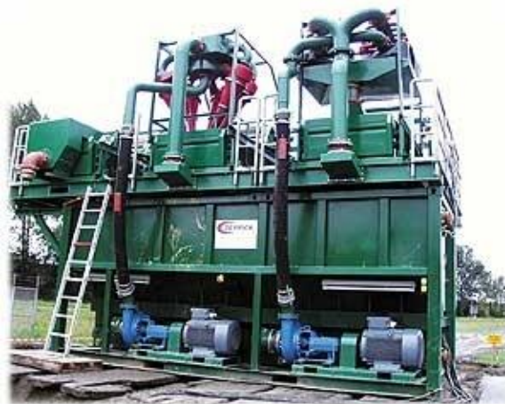
A typical microtunnelling spoil separation and fluid recycling set-up. Picture courtesy of Derrick Corporation
