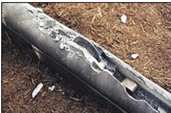
Above: A typical pipe splitting head assembly with cutter blades at the front followed by the expansion shell. Left: A pipe splitter unit 'cutting' a ductile pipe material.
